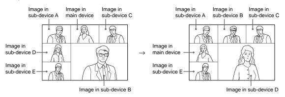
4. The splitting position can be fixed during six-image splitting. When "splitting (Fix A)" to "splitting (Fix E)" or "Splitting (Fix the local side)" is selected in a main terminal, the image in the selected terminal moves to the lower-right position and the image in a main terminal moves to the position of the selected terminal.
